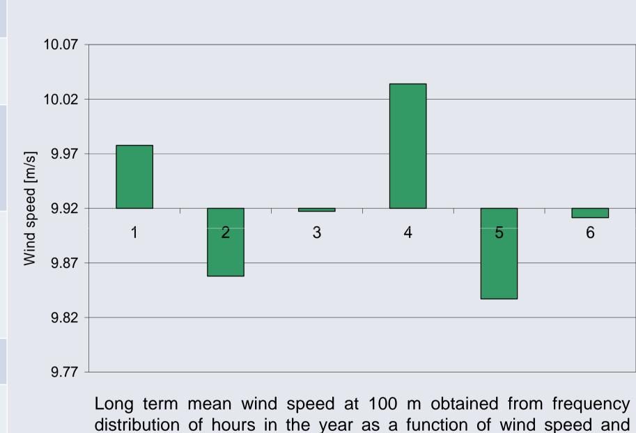
**3.Vertical extrapolation**: everybody has used the Hellmann exponential law that has good results for annual mean values but no when profiles are classified in terms of the observed atmospheric stability and, where the wind shear is overestimated during unstable conditions and underestimated in stable conditions. Stability and how it could be applied for wind resource assessment estimation should be analyzed.
